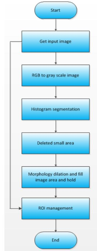
Fig. 2. ROI (cloud) automatic detection based on histogram segmentation algorithm.
